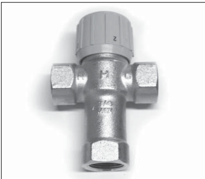
Figure 19 - Adjust Thermostat Mixing Valves at each point-of-use to 120°F (49°C) or lower.
